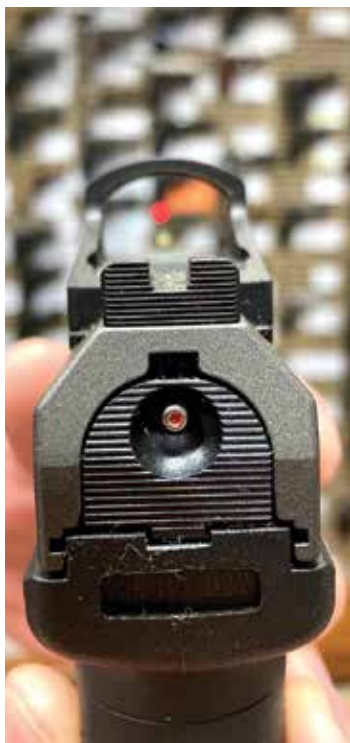
Co-witness capability compensates for a potential shortcoming of electronic handgun optics.
