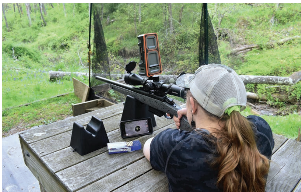
Serena is using the Longshot LR-3 two-mile system to sight in a .22 LR at 200 yards. This system makes it possible to see and mark impacts on the corresponding Longshot app. (Photo: Max Crotser)
